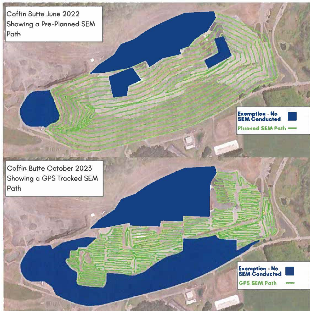
Figure 4 - Planned SEM route Differs Greatly from Actual SEM route
